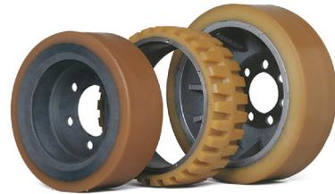
Electric pallet trucks and stackers only have solid tyres, because they are mainly used indoors and on flat surfaces.
