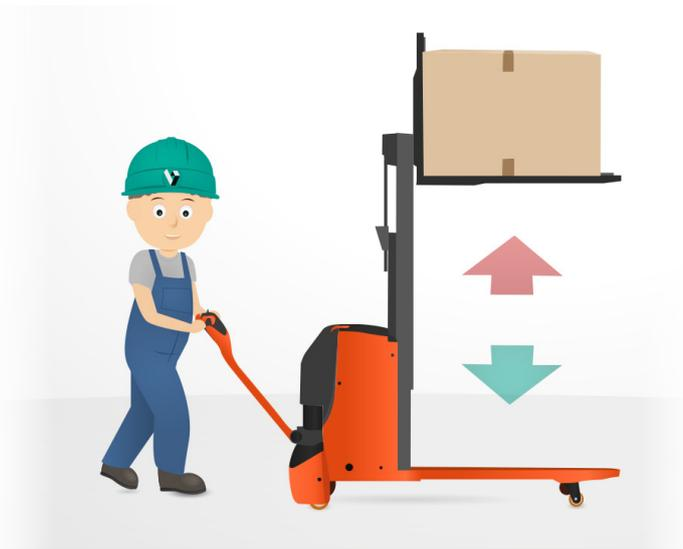
The first six factors have an adverse effect on the stability of the electric pallet truck or stacker, with or without load, due to the so-called lever effect. These factors will be discussed and explained later. The final two factors are related to adverse forces caused by driving the electric pallet truck or stacker at a certain speed.
